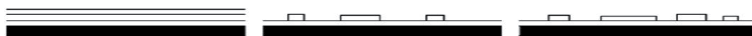
Figure 1. Illustration of the three different growth modes. Left: FM growth. Center: SK growth. Right: VW growth.
