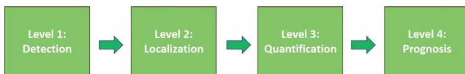
Figure 2. Schematics of the four SHM levels established by Rytter et al.
