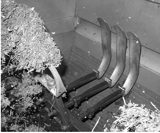
Figure 12. Tea-rolling machine. From Sayama cha no seisan yōgu: Hōkokusho (Iruma: Iruma Museum, 2009), p. 24.
