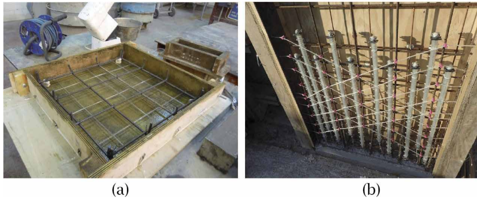
Figure 10. (a) Vascular network in concrete slab panel and (b) vascular network combination with PET in field trial (Reproduced from [56]).
