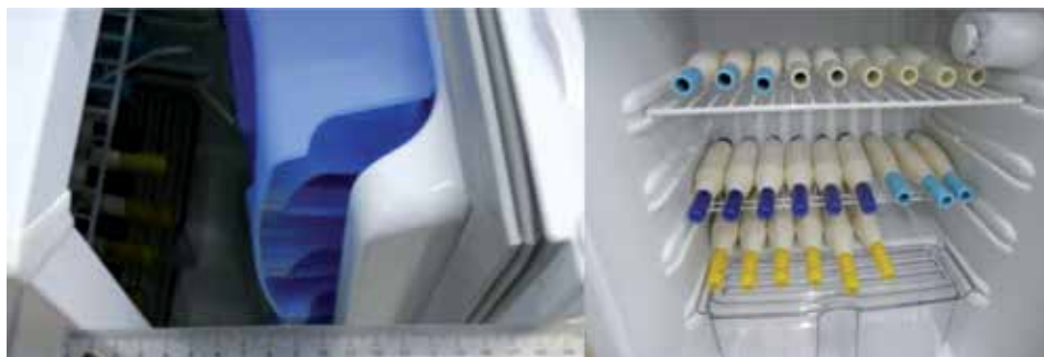
Figure 2. Refrigerator with the door opened in 8 cm and bobbins inside the refrigerator. Source: Author
