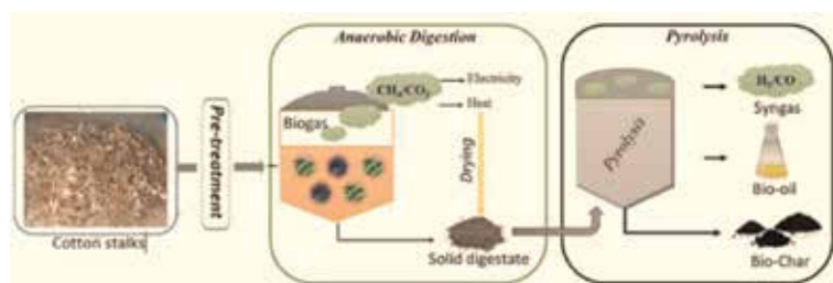
Figure 8. The system boundary of coupling anaerobic digestion and pyrolysis process.
