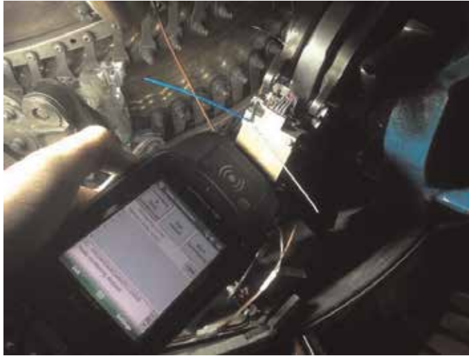
Figure 12. Reading distance with dipole antenna.
