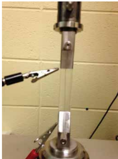
Figure 5. Composite sample mounted on test frame for mechanical test. Sensor lids are connected to the oscilloscope.
