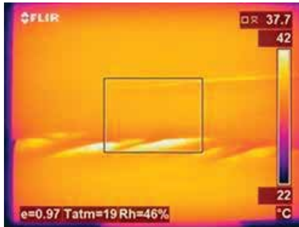
Figure 4. Thermogram of a wood sample with visible cracks (active method).
