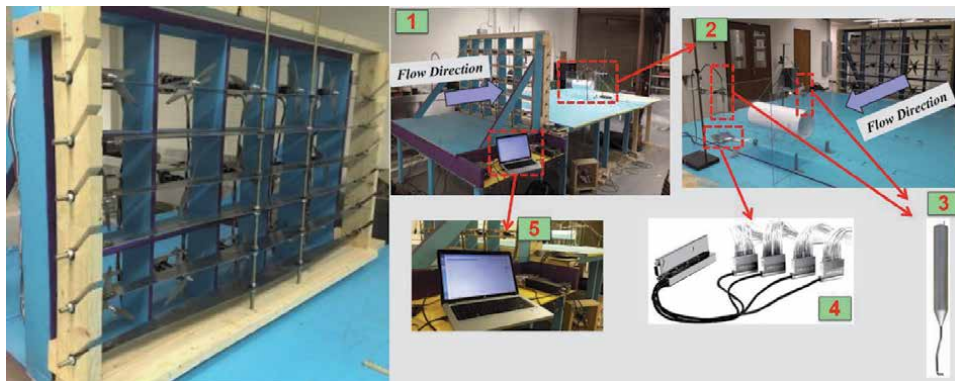
Figure 9. LSU WISE small open-jet hurricane simulator (with adjustable turbulence and profile production mechanism): (1) general view of testing setup, (2) section model test specimen, (3) cobra probes for measuring 3-component wind velocities, (4) ZOC23b miniature pressure scanner, and (5) laptop computer with software for data collection and processing.
