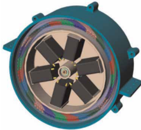
Figure 32. DFIA design with built-in rechargeable batteries.
