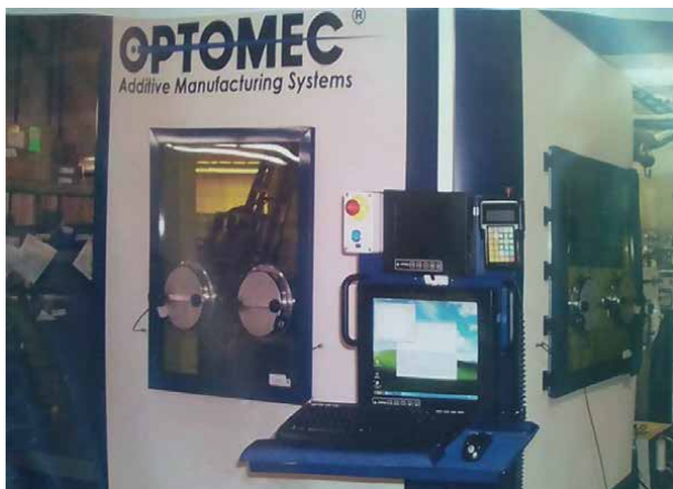
Figure 4. LENS Optomec 850R additive manufacturing system.
