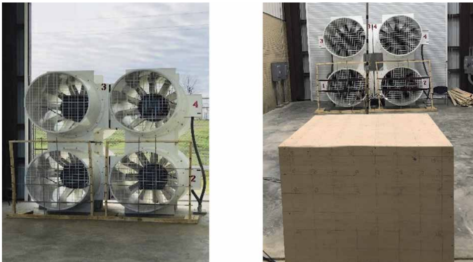
Figure 10. LSU WISE large testing facility (with a test section of 4\text{ m} \times 4\text{ m} ).
