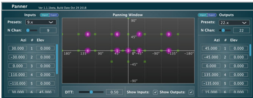
Fig. 3.12 The Panner VST plug-in from Aalto University’s SPARTA plug-in suite manages Vector-Base Amplitude Panning within sequencers supporting VST
