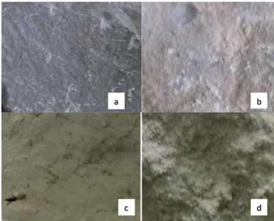
Figure 1. (a) Marly shale, (b) Şırnak limestone, (c) Şırnak porous limestone, and (d) the chemically degraded porous limestone.
