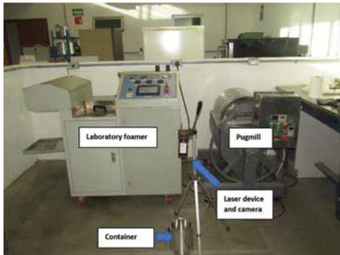
Figure 1. Laboratory test setup for measuring binder foaming characteristics (Lasfalto Laboratory, 2018).
