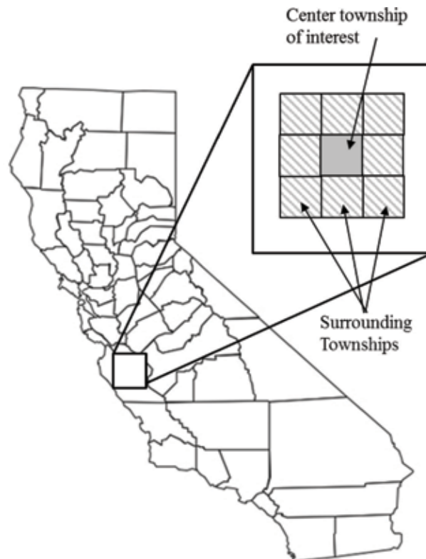
Figure 3. Example of a 3 \times 3 township air shed for SOFEA simulation from the state of California.
