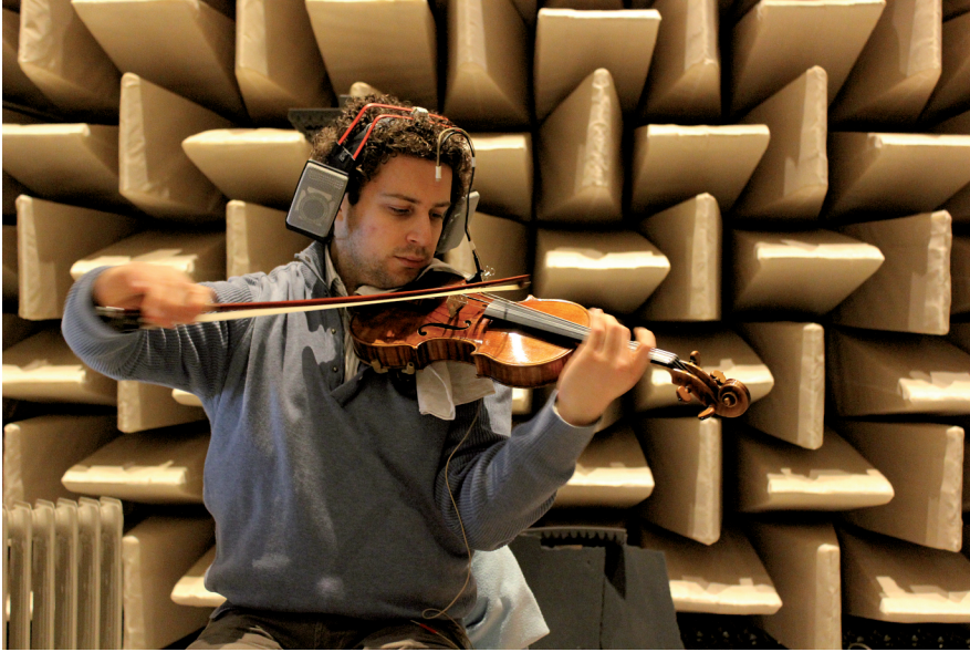
Fig. 3: Violinist playing in an Augmented Reality with extra-aural headphones. The direct sound of his instrument, unobstructed by the open headphone design, is mixed with the simulation of a concert hall, generated by binaural synthesis. 2
