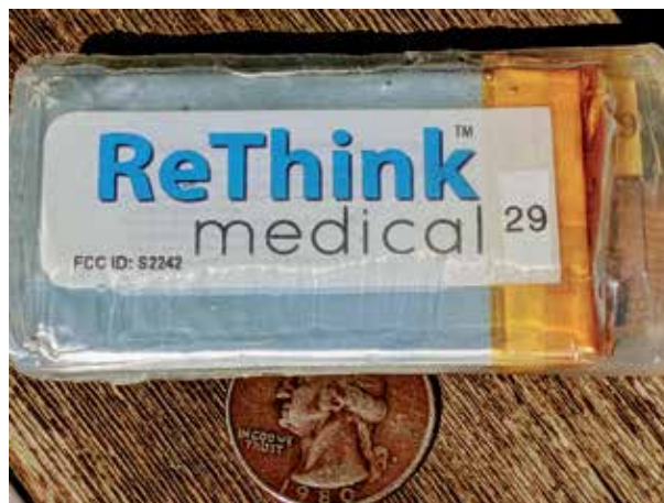
Figure 1. ReThink wireless biosensor with capability to acquire HR, three-dimension accelerometry and respiration data. These data are then transferred to a Bluetooth enhanced personal device, as well as stored there. Quarter is shown for size comparison, with dimensions of 7.5 mm width, 4 mm height, and 1.4 mm depth (used with permission).
