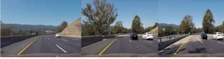
Figure 1. Image samples used in the study. Images contain distortions that are caused by lane boundaries of various colors, different environmental aspects, and change of road color that is caused by various light conditions and color differences which all push the model to make errors.
