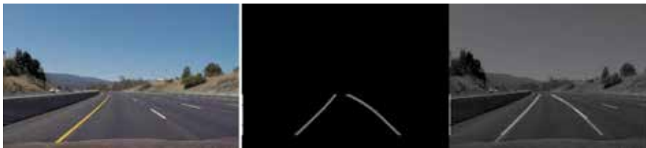
Figure 7. Plot fitting example. Original image (left) went through the process covered in recent subsections. For found center lane boundaries, we fit a plot with the normal equation method which is covered in this subsection. Two-line image (middle) found as output and finally added to the grayscale version of the original image for comparison.
