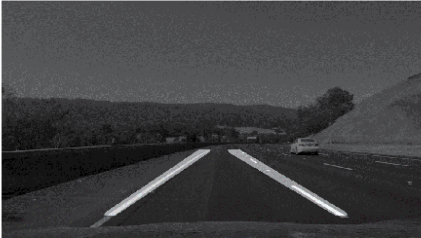
Figure 6. Region of interest to be used in the next frame. After Hough transform, we have exact locations and orientations of center-lane boundaries. A region of interest is specified according to this information and the process is applied only within the region of interest. The image above is the sum of the region of interest and grayscale version of the original image.
