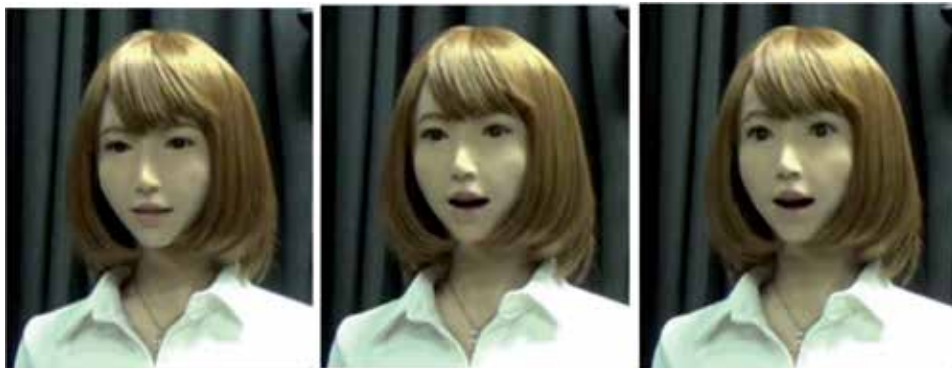
Figure 4. Examples of generated facial expressions for eyebrow and eyelid control at level 0 (neutral idle face, left), level 1 (slight surprise face, middle), and level 2 (clear surprise face, right).
