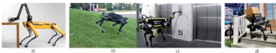
Figure 3. Robotic quadrupeds. (a) SpotMini [13], (b) Laikago [14], (c) ANYmal [15], (d) ANYmal and Continental [16].
