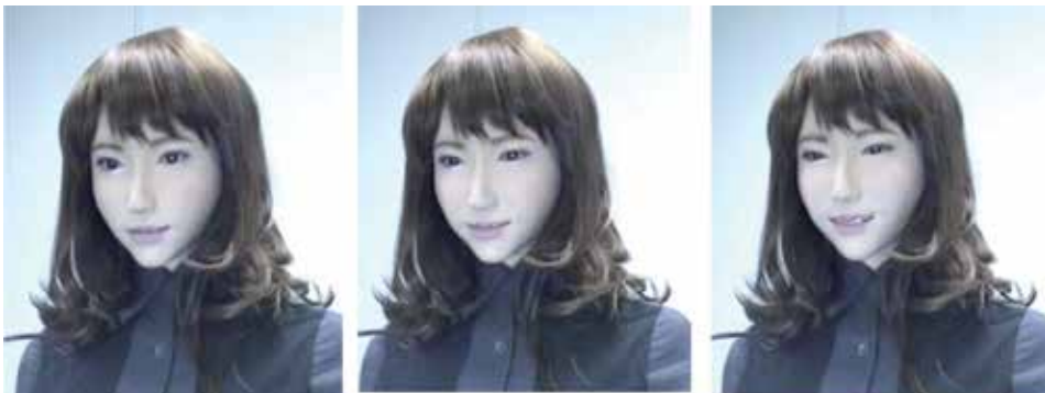
Figure 3. Examples of generated facial expressions by eyelid and lip corner control: neutral face (left), idle slight smile face in non-laughter intervals (middle), and smile face during laughter intervals (right).
