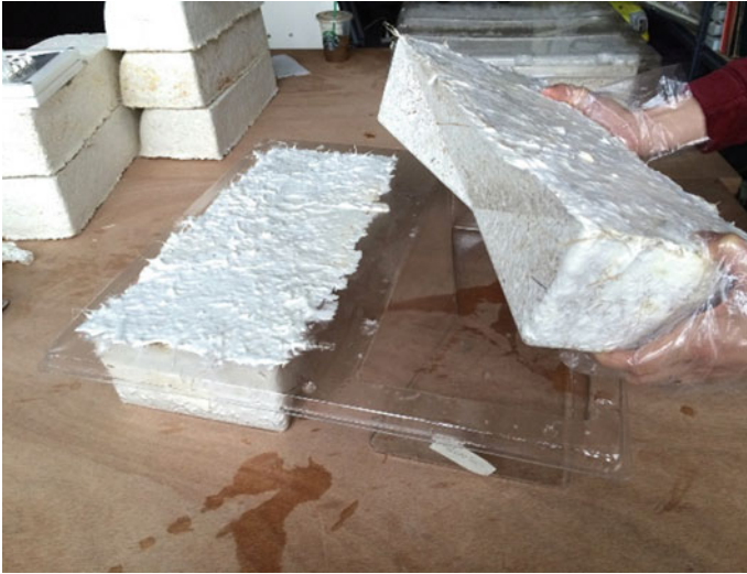
Fig. 3.2 Bricks made of fungal mycelium. Image courtesy of The Living
