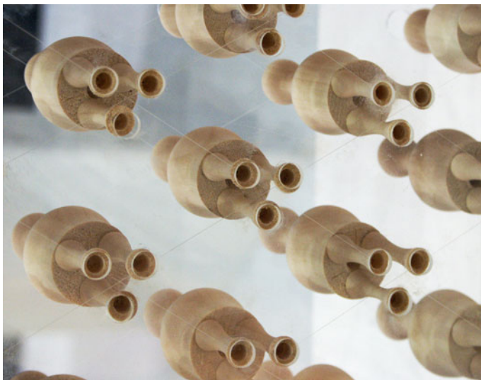
Fig. 1.9 Conceptual façade system modelled on the principle of gaseous exchange in insects. Picture taken during Glasstec Messe 2004, Glass Technology Live Show, Institute of Building Technology and Design, Stuttgart, Prof. S. Behling, Dr. Henning-Braun
