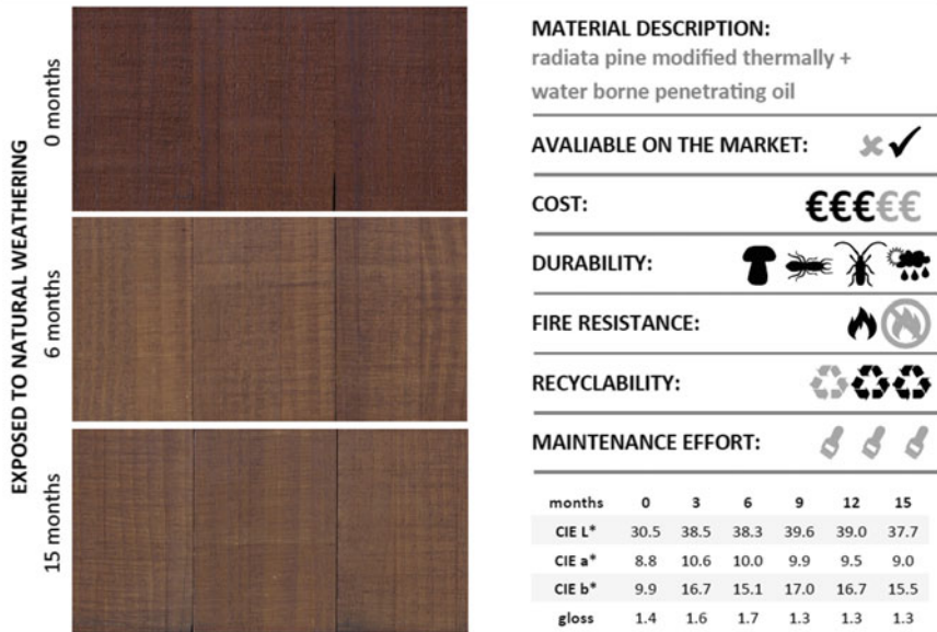
Fig. 6.23 Technical characteristics of TM pine impregnated with oil
