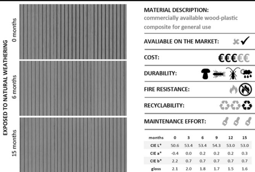
Fig. 6.30 Technical characteristics of wood-plastic composite
