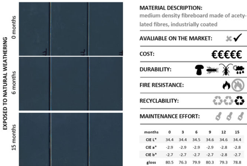
Fig. 6.29 Technical characteristics of fibreboard made of acetylated fibres
