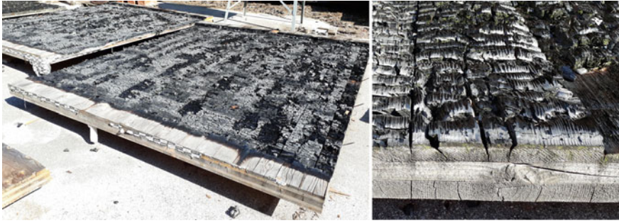
Fig. 3.23 Carbonized surface of the CLT panel after fire test preserving structural integrity of the wall
