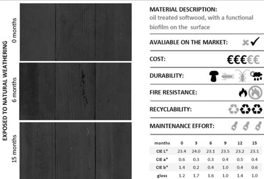
Fig. 6.26 Technical characteristics of biofinished pine
