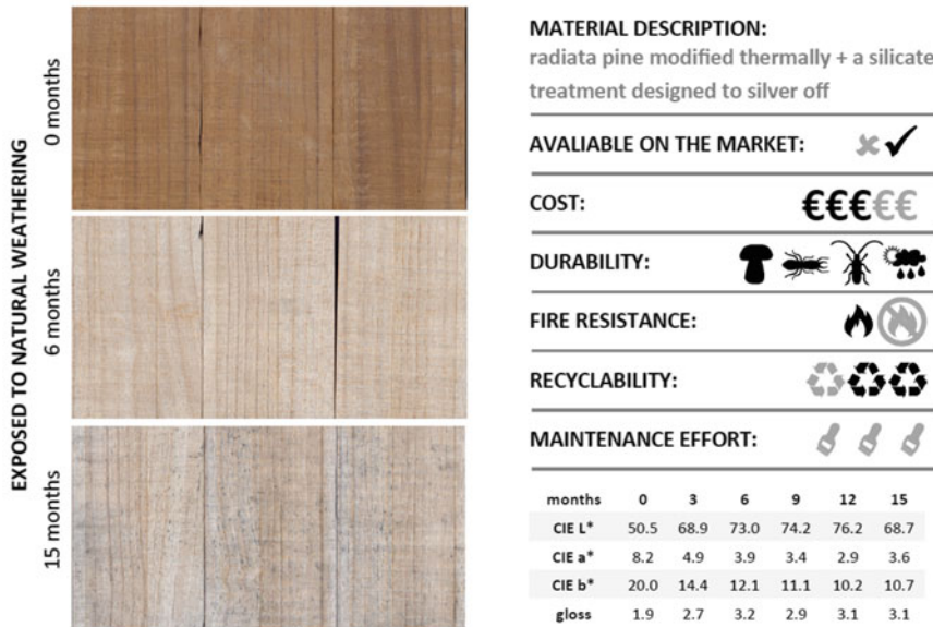
Fig. 6.24 Technical characteristics of TM pine impregnated with silicate
