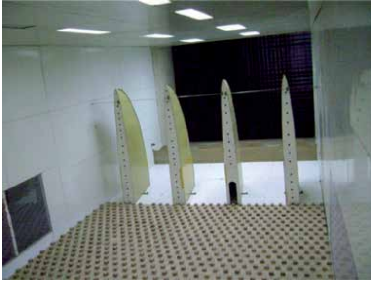
Figure 4. Counihan vortex generators, barrier, and roughness elements of the full-depth boundary layer simulation.
