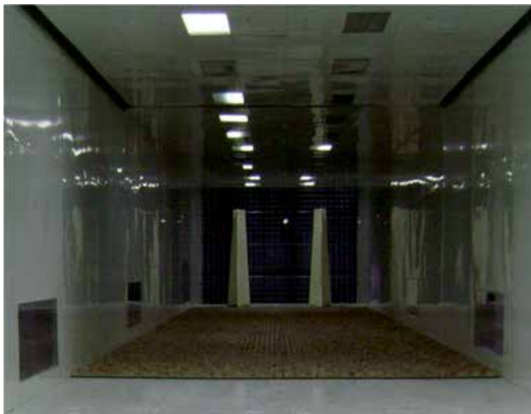
Figure 7. Irwin vortex generators and roughness elements of the part-depth boundary layer simulation.
