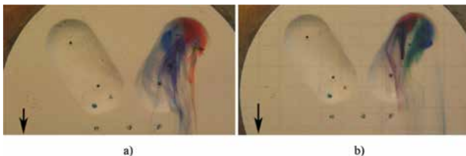
Figure 3. Flow visualization inside the oval dimple for Re_x = 48,000 (a) and Re_x = 96,000 (b).
