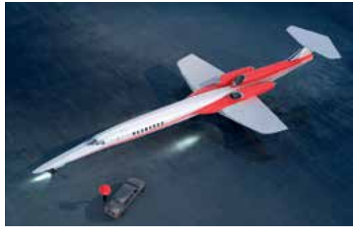
Figure 2. Low-sweep Aerion AS2 supersonic Bizjet. M_\infty \leq 1.5 . Posted by Tim Brown on the Manufacturer Newsletter.
