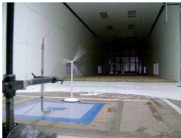
Figure 20. Wind turbine model spinning during the wind tunnel test.
