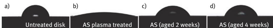
Figure 2.9: Evolution of the contact angle of an ASP-treated carbon surface with time. Reprinted with permission from [30]. Copyright 2017, American Vacuum Society.
