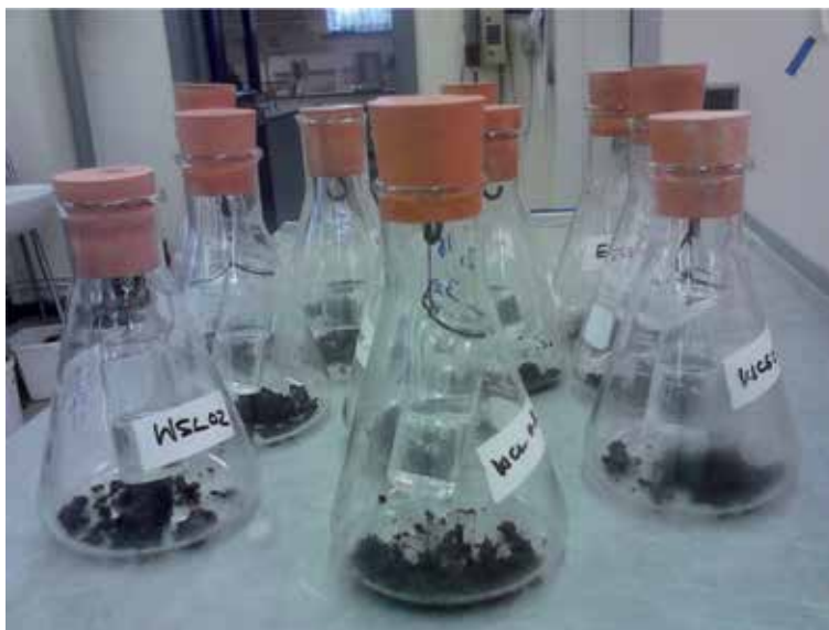
Figure 1. Photograph of CO 2 -C emission experiment.
