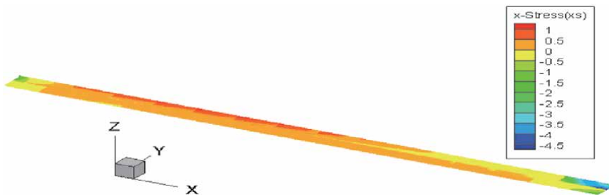
Figure 15. Contour of the dam axial stresses of the connecting plate and toe slab during the storage period (MPa).
