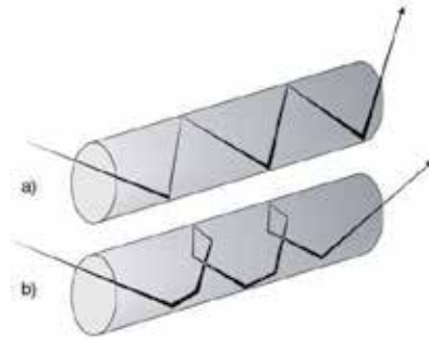
Figure 13. Rays taking meridional (a) and helical (b) forms in an optical fiber [12].
