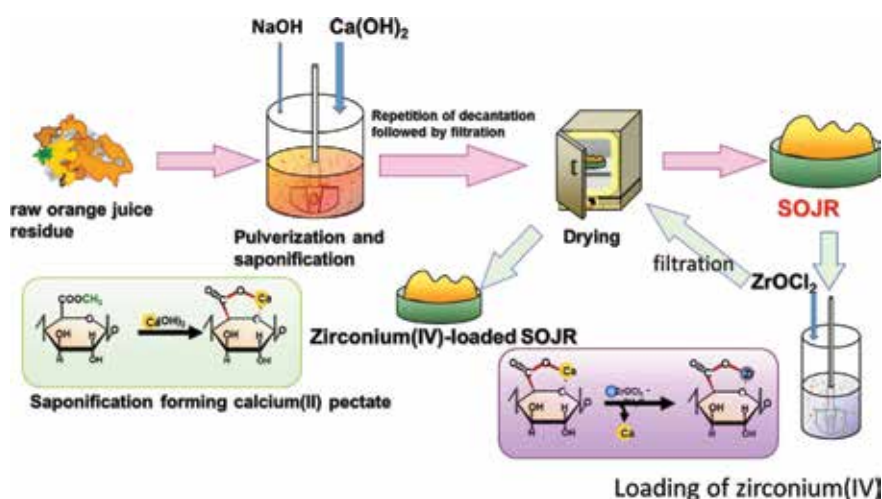
Figure 4. Preparation route of adsorption gels from OJR.
