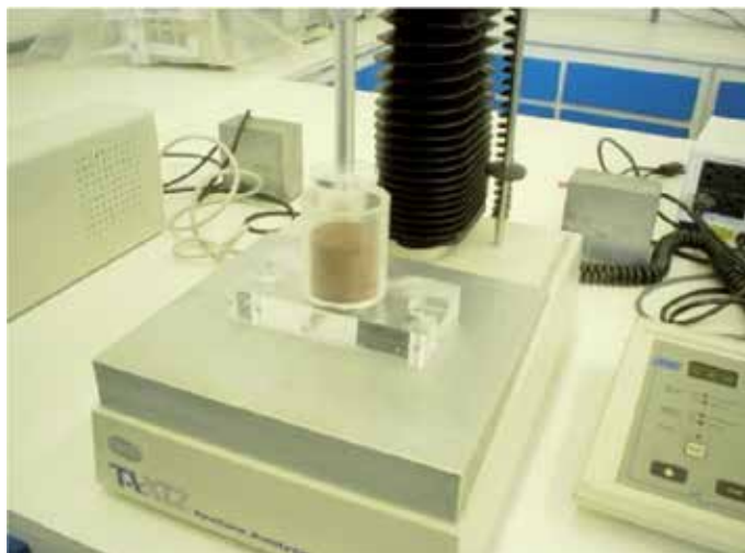
Figure 3. Texturometer, back extrusion probe and cylindrical cup with sample.
