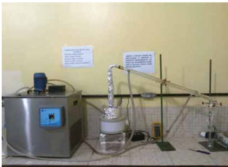
Figure 2. Vigreux borosilicate-glass distillation column of 500 ml, electrical heating mantel, cryostat bath, Liebig condenser, and separating funnel.
