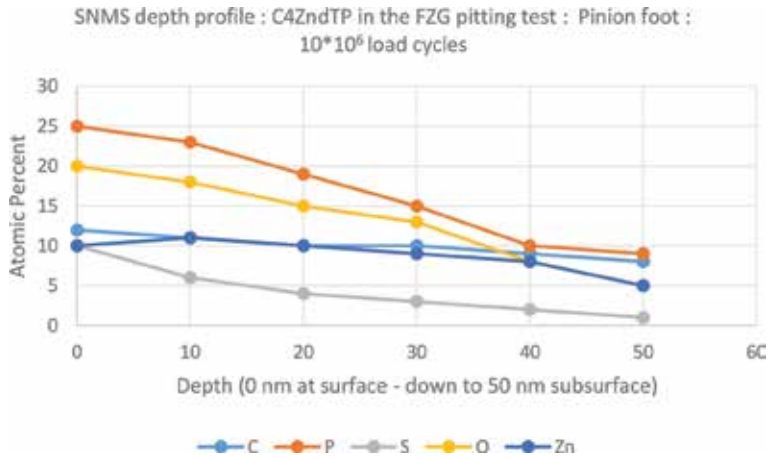
Figure 10. SNMS depth profile: C4ZndTP in FZG pitting test at 10 \times 10^6 load cycles.
