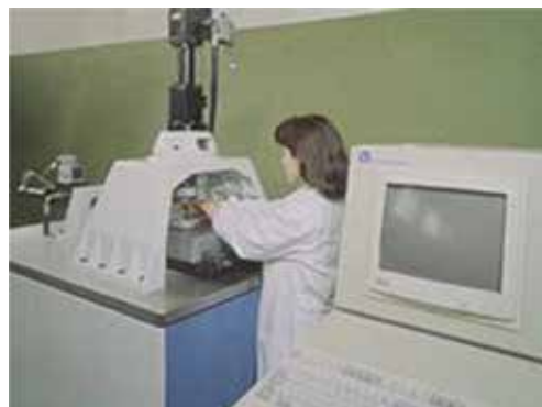
Figure 5. Plain bearing testing machine, designed and constructed by TEKNIKER for Mecauto-Wisco company.
