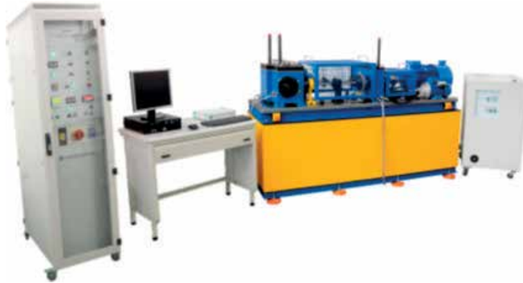
Figure 8. Photograph of the T-30 back-to-back bevel gear test rig with its control and measuring system (on the left) and water circulating cooling system (on the right) [44].
