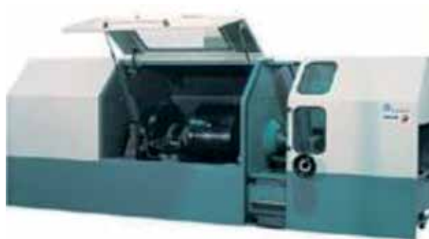
Figure 9. Disc brake testing machine, designed and constructed by TEKNIKER for Fagor Ederlan company.
