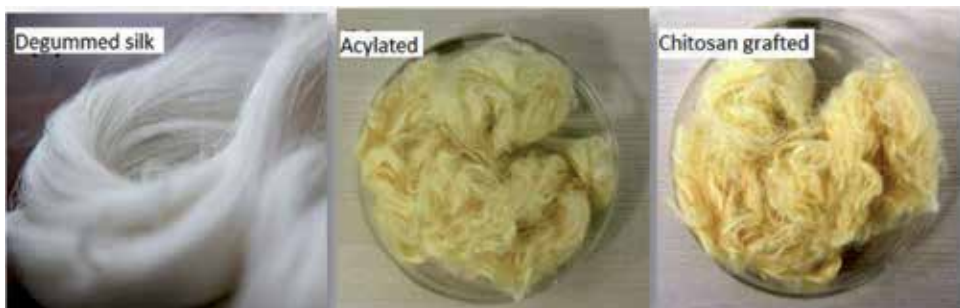
Figure 6. Image depicting degummed, acylated and chitosan grafted silk fibres.
