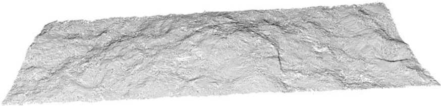
Fig. 5.17 Point cloud representing the surface of a granite sample from Saxony. The size is 65 mm by 170mm and the cloud contains approx. 98000 points
