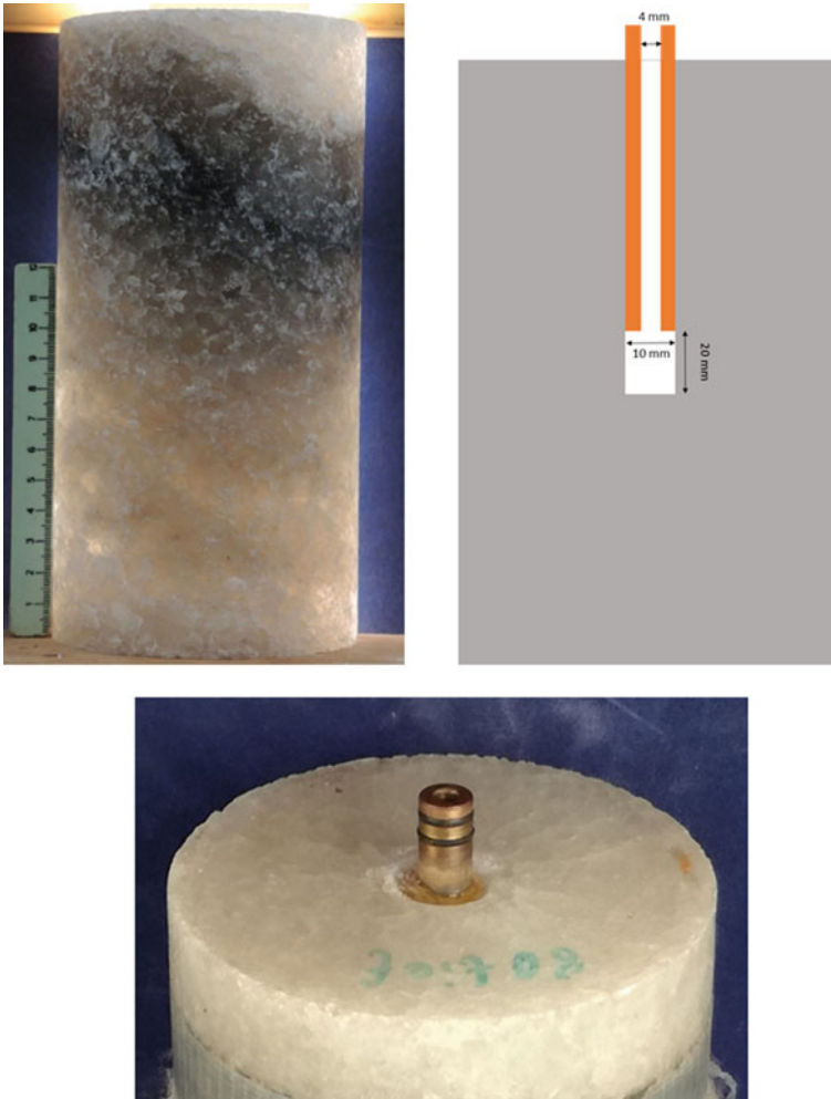
Fig. 4.69 Rock salt sample, borehole geometry, detail of metal pipe
