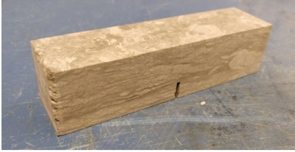
Fig. 2.18 The prepared Opalinus Clay sample with the dimension of 140 \times 30 \times 30 mm
