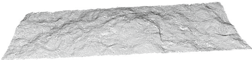
Fig. 4.86 Point cloud representing the surface of a granite sample from Saxony. The size is 65 mm by 170 mm and the cloud contains approx. 98000 points. The shear direction is parallel to the long edge in a way that the shown surface remains in its position and its top counterpart is moved to the right
