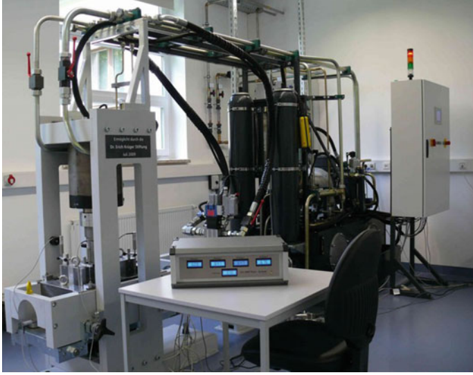
Fig. 2.36 The shear testing device at the rock mechanical laboratory of the TU Freiberg. (From: [36])
