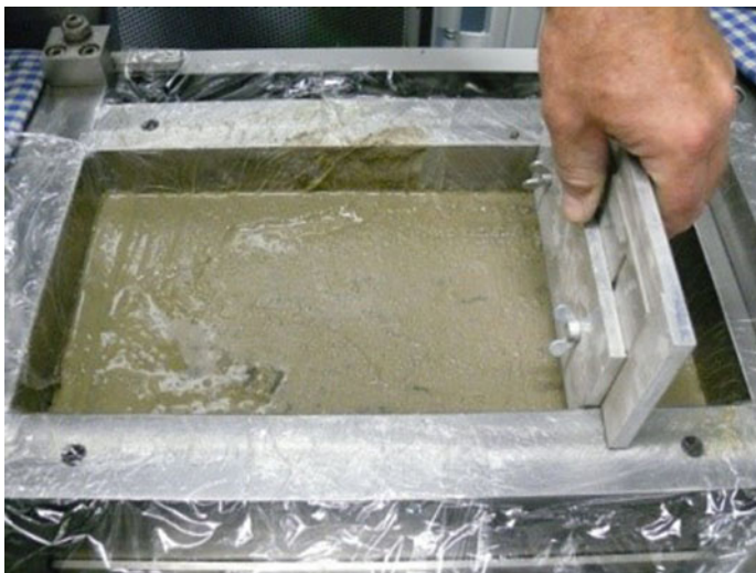
Fig. 2.38 Grouted sample before direct shear test (From: [37])
