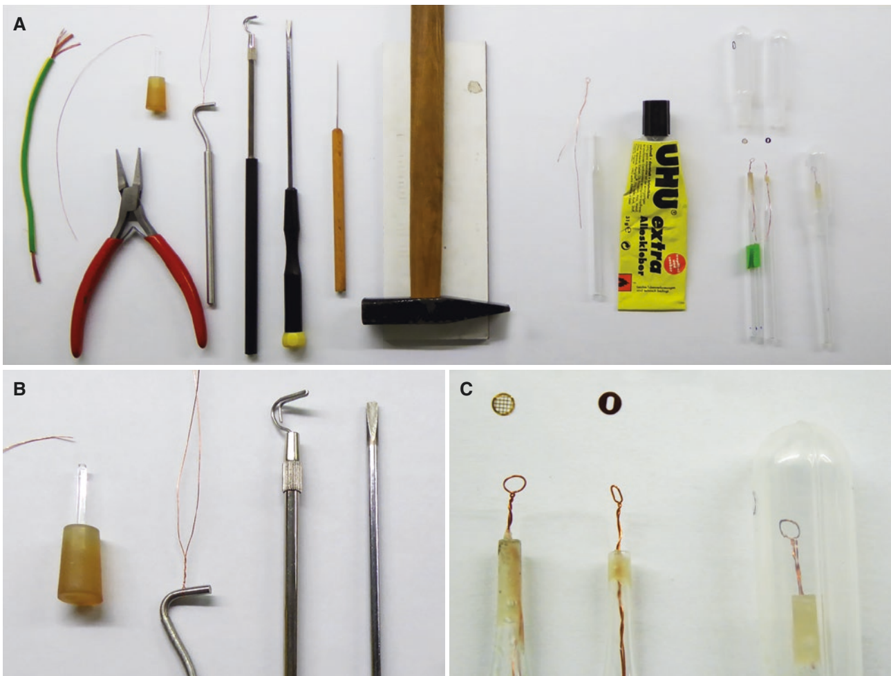
Fig. 15 Making loops. A. Technical equipment for making loops. B. Wire twisted around a circular object (model form) for mesh grids. C. Loops fixed with wax on glass pipettes (left), for storage loop covered with the back end of a disposable plastic pipette (right)
