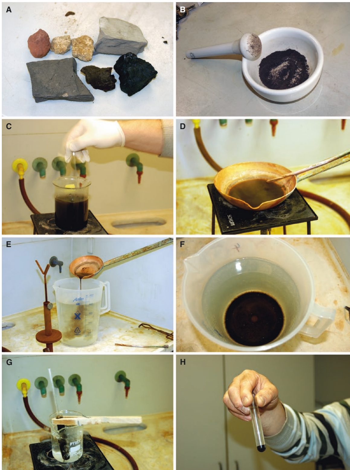
Fig. 23 From rock to palynomorphs. A. Different types of sedimentary rocks: reddish, yellowish, and white-greyish samples usually contain few and/or badly preserved palynomorphs (back row), brown, dark-grey to blackish samples often contain well preserved pollen (front row). B. Sedimentary rock sample (ca 30 g) hand grounded in a mortar with a pestle. C. Sample boiling in \geq 200 ml of HCl. D. Sample boiled in a copper pan with \geq 150 ml of HF. E. The HF solution is poured slowly into a large plastic beaker filled with water. F. Organic material settled on the bottom of the beaker. G. Acetolysis, test tube in boiling water, note the stirring glass stick. H. Acetolyzed sample before decanting of water following the final wash
