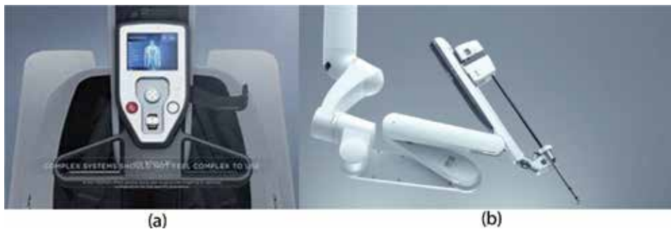
Figure 5. The patient cart. (a) The visual pad on the patient cart that allows operator to set the type of surgery to be performed and the handles that allows the patient cart to be moved around theatre. (b) A robotic arm with an instrument in place. The port and instrument clutches can be utilised to move the instrument into the correct position. Setting set-up it must be ensured that the robotic arms are in the correct alignment to avoid unnecessary collisions and clashes between arms.
