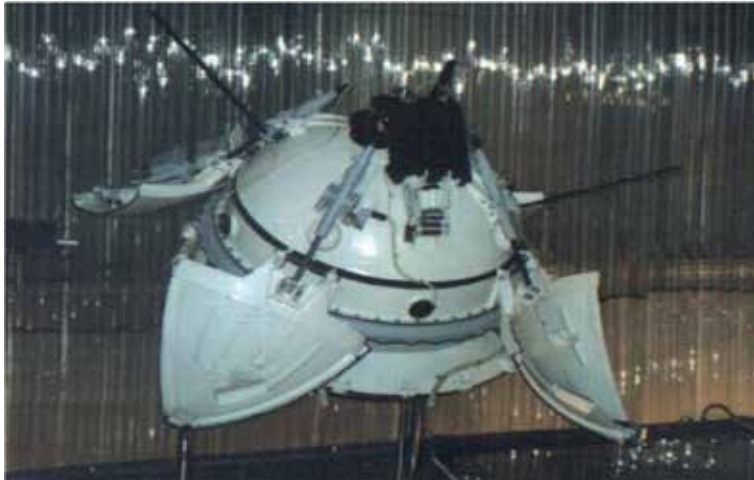
Figure 4. The Mars 3 lander. Credit: NASA [6, 7].
