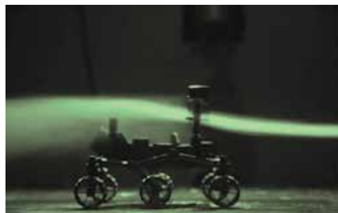
Figure 10. Smoke visualization of flow around rover ( Re = 2.2 \times 10^5 ).
