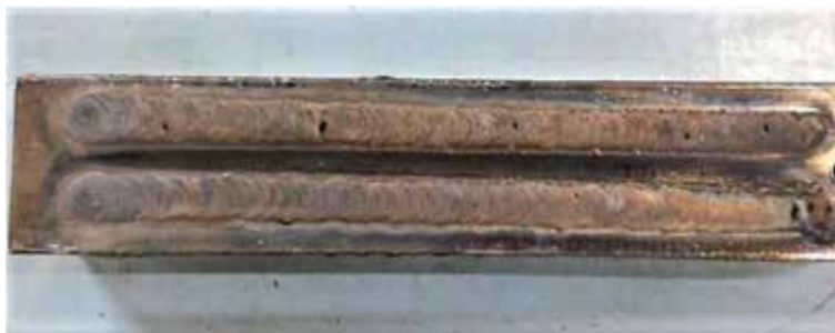
Figure 4. Cu-Sn alloy surface modified with Ni.
