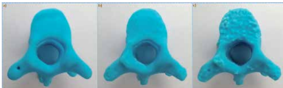
Figure 4. Results of each produced model. (a) Reference model, (b) Mean filter and (c) Smooth tool.
