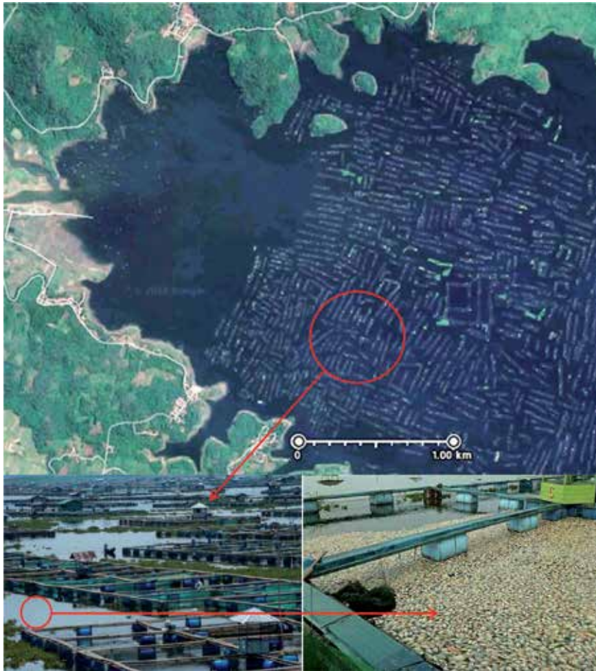
Figure 1. Aerial image of Cirata dam located in West Java, Indonesia (upper) showing uncontrolled density of floating cage aquaculture causing rapid degradation in its water quality (lower-left); deaths of thousands of tons of fish in floating cages aquaculture due to lack of oxygen and rising toxic gas (lower-right) causing economic loss of approx. USD 28.5 million [29]. Image courtesy of Google maps [31–33].
