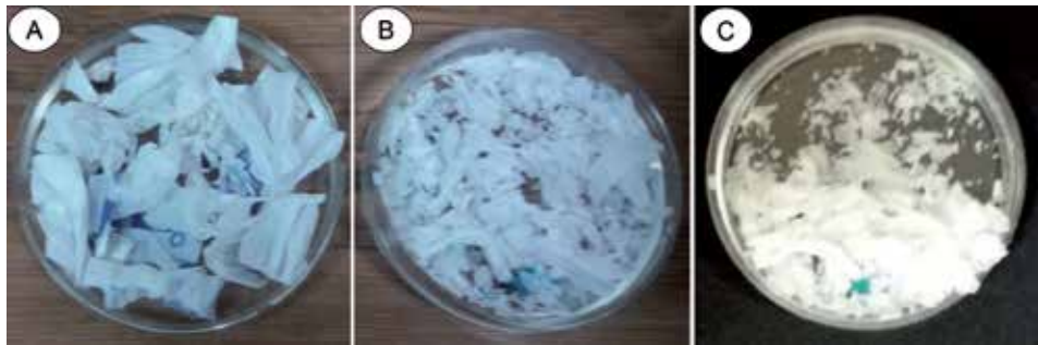
Figure 3. Oxo-biodegradable plastic bags before (A) and after 21 months of exposure to sunlight (B and C). The letter C shows the fragmented plastic.
