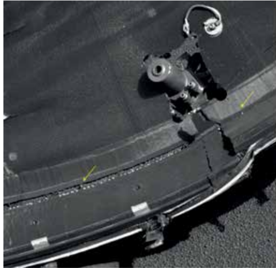
Figure 14. Evidence of fresh blueberries collected by heat shield. Image 1P158281536EFF40C2P2368L6M1 (sol 339). Image courtesy: NASA/JPL & M Lyle.
