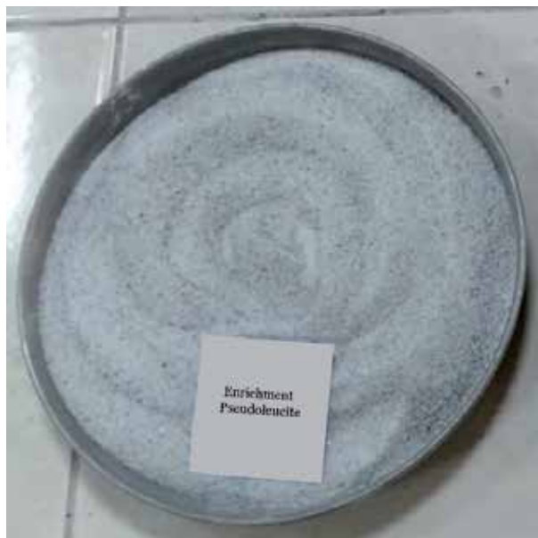
Figure 11. The appearance of the product obtained after magnetic enrichment.
