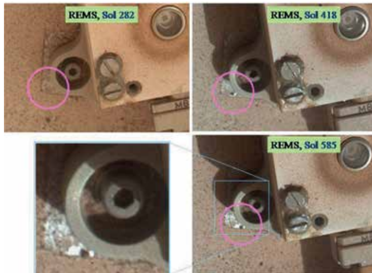
Figure 18. Images of REMS-UV sensor on Curiosity rover showing a cosmic spherule impact.
