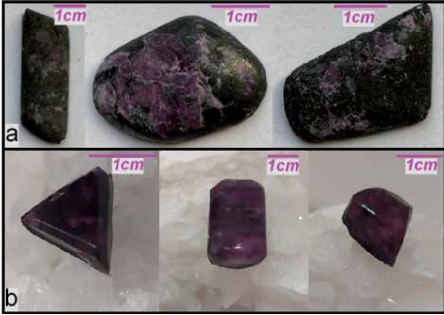
Figure 5. Gemstones made from kammererite samples taken from the study area (a—processed samples without treatment; b—processed samples after treated with epoxy).
