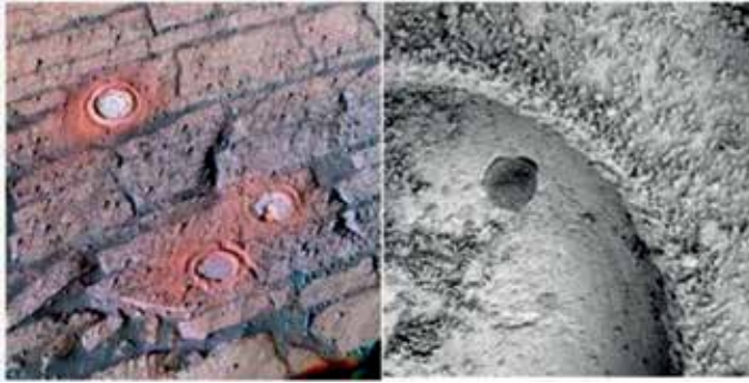
Figure 4. Rock abrasion tool (RAT) was used to cut some of the spherules embedded in the soil. The hematite spherules show no internal structure. (Image courtesy of NASA/JPL).
