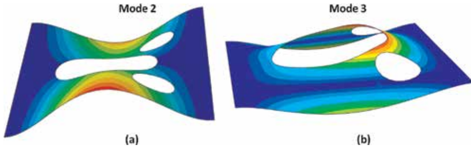
Figure 9. Mode shapes of the optimized structure shown in Figure 8 . (a) Lower Mode (Mode 2 of the structure) (b) Upper Mode (Mode 3 of the structure).
