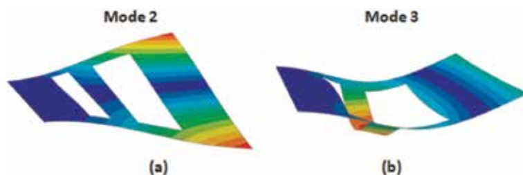
Figure 6. Mode shapes of the optimized structure shown in Figure 5 . (a) Lower Mode (Mode 2 of the structure) (b) Upper Mode (Mode 3 of the structure).
