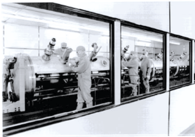
Figure 3. Working to protect the Q of superconducting cavities. Four-cavity module for LEP being equipped with HOM and power couplers in a class 100 clean room [29]. Any impurity at the level 10^{-9} would produce heat spots, while the cavities operate to deliver, of the order of 500 Gev energy to the passing electrons.
