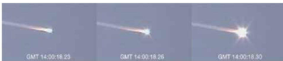
Figure 20. Acceleration phase of the destruction process (phase A) [25].
