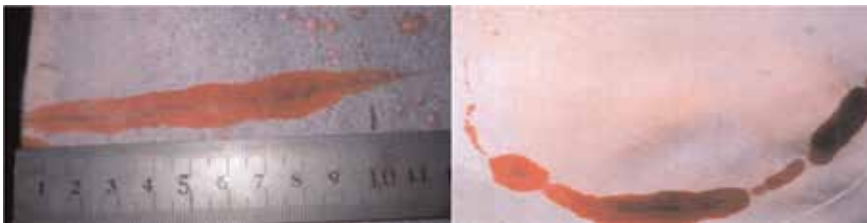
Figure 4. Cracks in metal of impeller blades.
