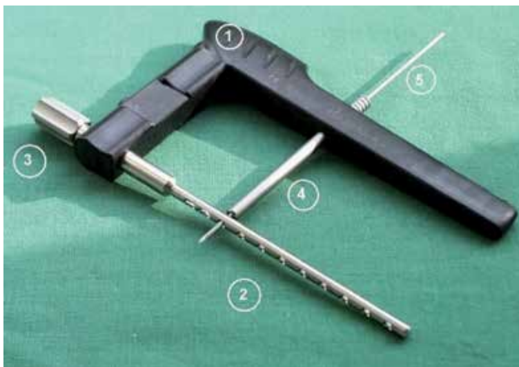
Figure 11. Standard XS nail with aiming device: (1) X-ray transparent carbon aiming device; (2) XS standard (4–5 mm) nail, here 12-hole nail; (3) adapter for the nail on the aiming device; (4) lateral drill sleeve for the locking wires; and (5) cross-locking threaded K wire.
