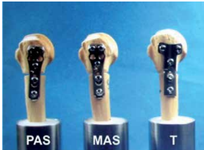
Figure 27. Sawbones with polyaxial angular stability (PAS) plate, monoaxial plate (MAS), or classic T plate (T).
