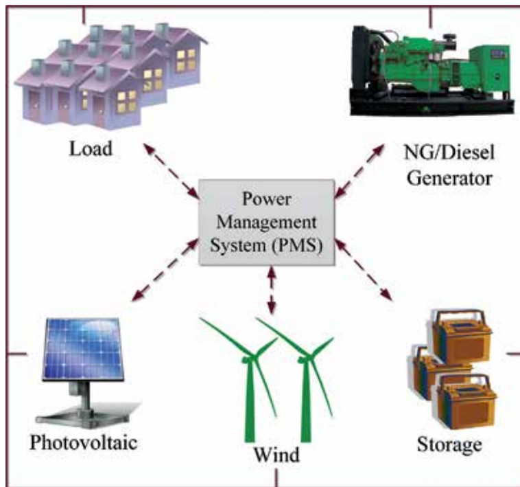
Figure 2. Microgrid and its components.
