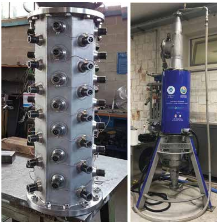
Figure 2. The inner part of the sono-heat-exchanger (on the left). The external structure of the sono-heat-exchanger (on the right).
