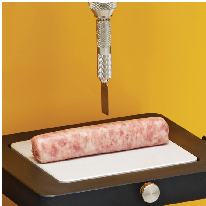
Fig. 2. The Brookfield Amatek Texture Analyser at work on a sausage. Courtesy of Brookfield Amatek.
