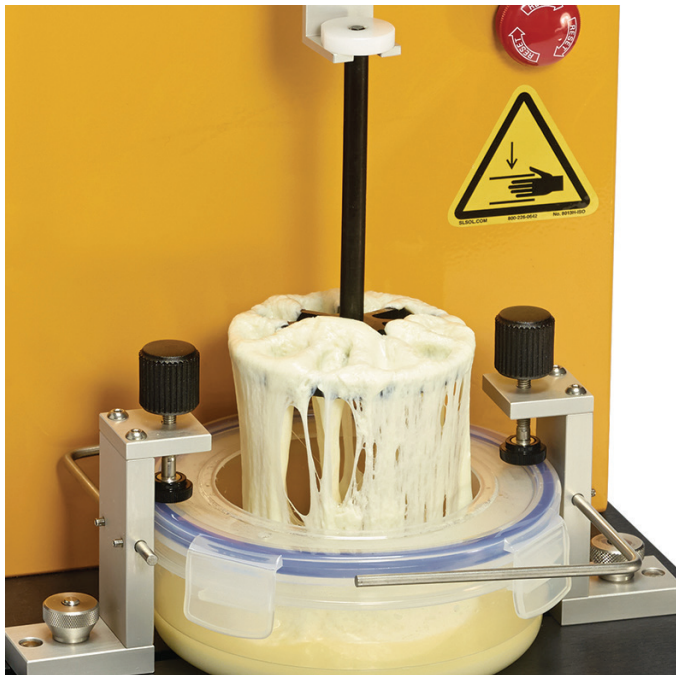
Fig. 4. The Brookfield Amatek Texture Analyser at work on some mettle cheese. Courtesy of Brookfield Amatek.
