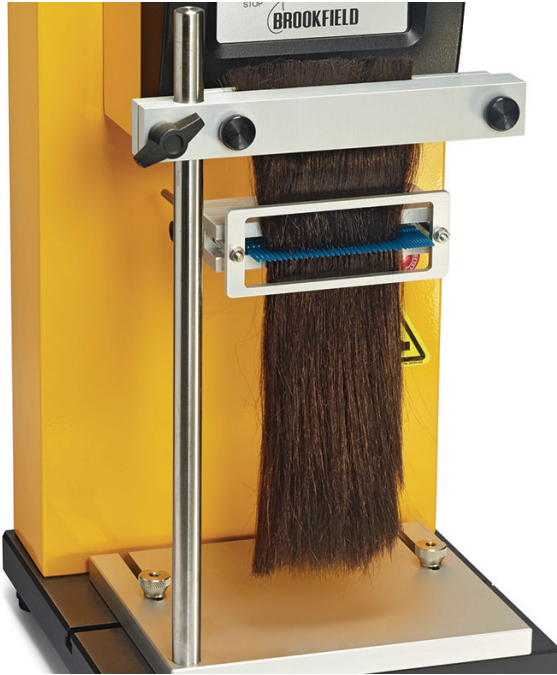
Fig. 5. The Brookfield Amatek Texture Analyser at work on a length of hair. Courtesy of Brookfield Amatek.
