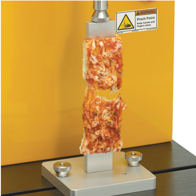
Fig. 3. The Brookfield Amatek Texture Analyser at work on a pizza. Courtesy of Brookfield Amatek.
