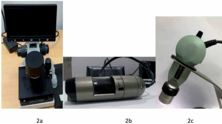
Figure 2. Various instruments used in nail fold capillaroscopy; (a) stereomicroscope, (b) microscope and (c) nail fold videocapillaroscope.
