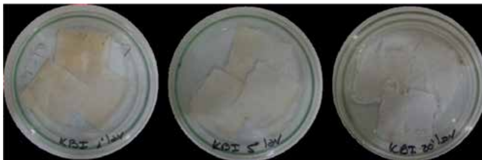
Figure 5. Photographs of the fabric with KBI after a first wash cycle (left), 5 wash cycles (center), and 20 wash cycles (right).
