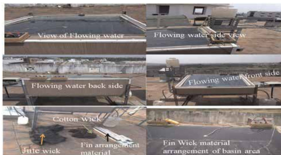
Figure 4. View of experimental works of water flowing over glass cover used by a solar still with absorbing materials.
