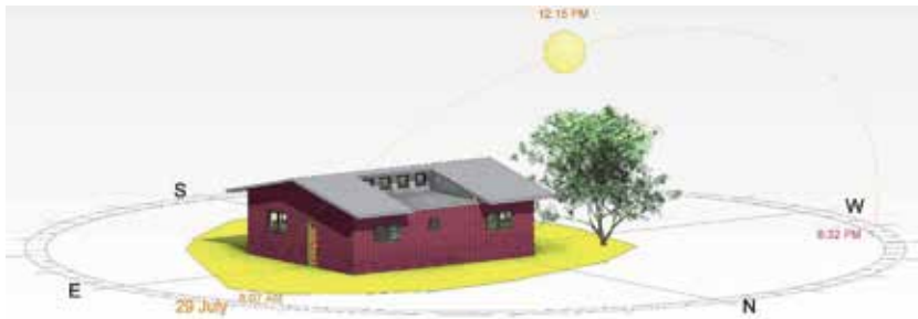
Figure 2. A 3D view sun path simulation of the house.
