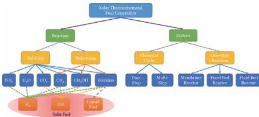
Figure 3. Classification of solar thermochemical fuel generation.
