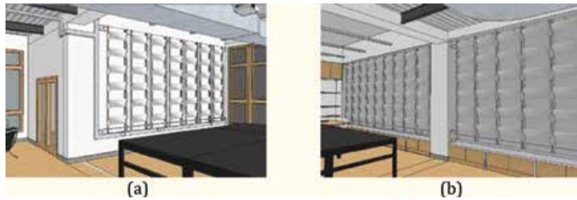
Figure 16. (a) Design sketch, PCM panel exposed to indoor air; and (b) design sketch, PCM panel decorated with perforated aluminum plate.
