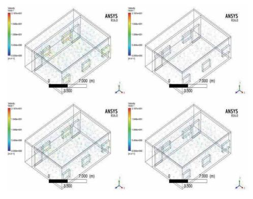
**Figure 13.** Velocity vector of air in the mechanical lecture room at different inlet velocities (0.05 TRH, 0.5 BRH, 1.0 BLH and 2.0 TRH m/s).
