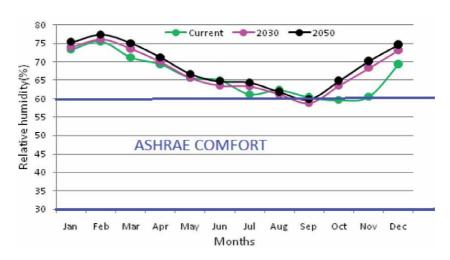
Figure 3. Monthly relative humidity in the new building during three periods (present, 2030 and 2050).
