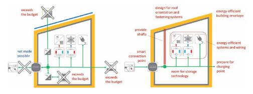
Figure 1. Zero-emission-ready building design.
