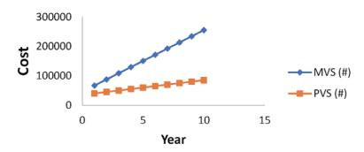
Figure 16. Graph of the cost of solar chimney and fans against number of years.
