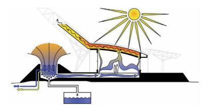
Figure 14. Hawaii Gateway Center radiant roof system.
