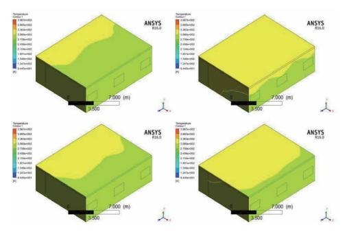
Figure 14. Temperature contour of air in the mechanical lecture room.
