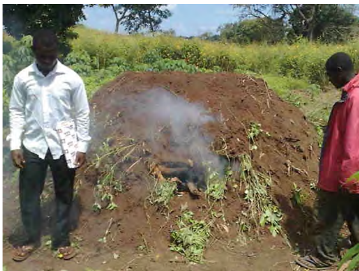
Fig. 2 Image of the combustion process during charcoal production in Saki from a field study conducted on April 19, 2013
