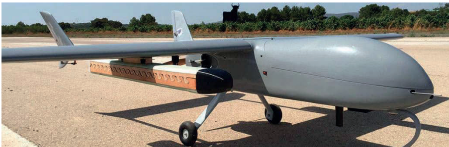
Figure 4. Unmanned aircraft developed for the Southern Tsetse Eradication Project in Ethiopia. The pods under the wings carry the sterile tsetse males in chilled conditions.
