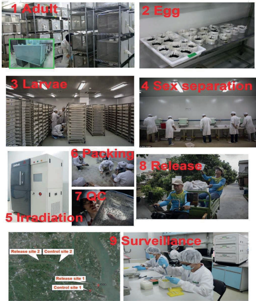
Figure 3. The different stages of the first combined IIT/SIT field trial against Ae. albopictus in Guangzhou, China. Photographs illustrating the nine different stages of the combined IIT/SIT field trial. In stage 1-3, artificially-triply-Wolbachia-infected adults, eggs and larvae were mass-produced in the mosquito rearing factory. In stage 4, a Fay-Morlan sorter was used for sex separation of pupae, followed by stage 5 with the Wolbaki® X-ray irradiator custom-made for the field trial to enable pupal irradiation. In stage 6, the sex-separated males were packed into buckets for mass-release. After quality control of emerged adult males by manual checking for contaminant adult females (stage 7), those buckets were delivered by vehicle to release sites (stage 8), as shown in the satellite images of the control and release sites (map data: Google, DigitalGlobe). Field populations were monitored through samples collected each week for diagnosis of wPip infection using PCR (stage 9).
