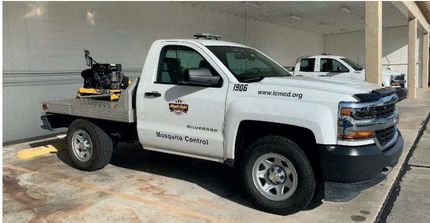
Figure 11. Ground adulticiding vehicles with rear-mounted ULV machine.
