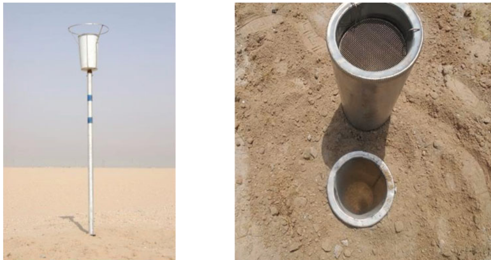
Fig. 7.1 Dust tarp fixed at 240 cm above ground level (left), and pollen traps before and after fixing (right)
