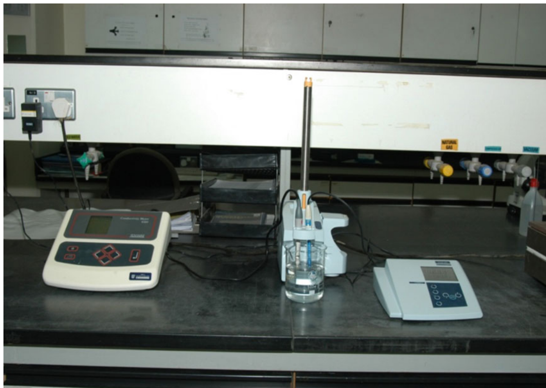
Fig. 8.2 Conductivity and pH meter used for dust samples
