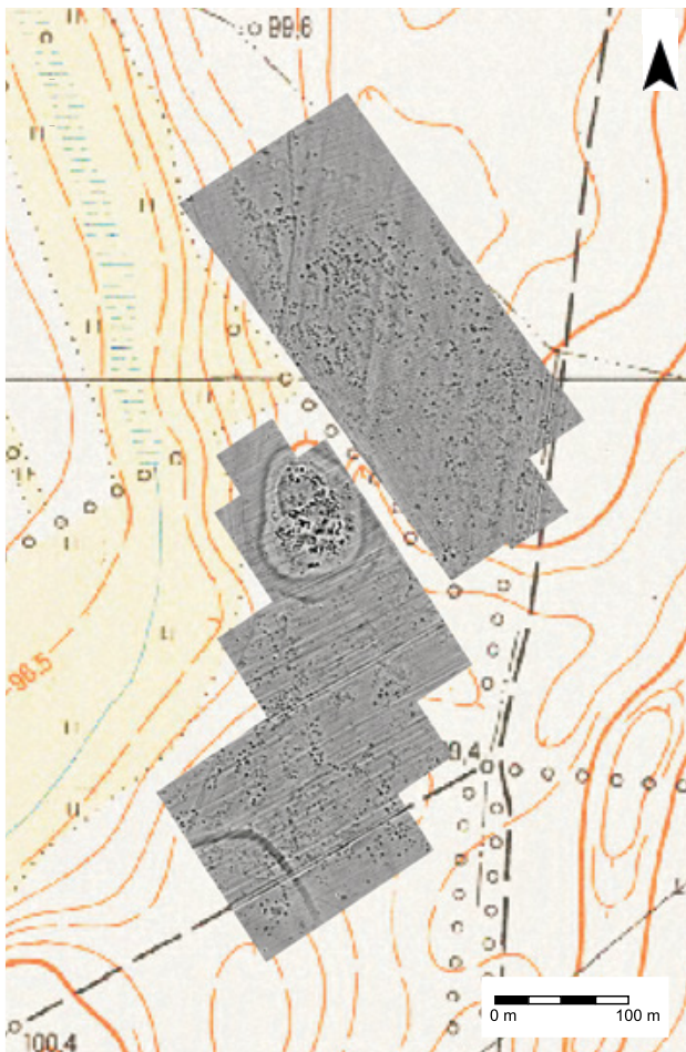
FIG. III-108: SZAKÁLD-TESTHALOM. MAGNETOMETER DATA OF THE CENTRAL TELL PART OF THE SITE AND THE MULTI-PHASE OUTER SETTLEMENT (GREYSCALE PLOT; DATA RANGE [BLACK TO WHITE]: +/- 10 NT).
